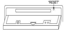
The RESET button is located on the front of main panel. It is recessed in order to prevent accidental engagement, and can be activated with the tip of a ball-point pen or any similar pointed object. This reset circuitry is provided in order to protect the unit's microprocessor, and should only be activated under the following conditions:
